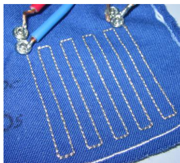
Figure 3.7: Test vehicle: the embroidered track has been embroidered three times one over the other (the same track) with Shieldex in needle and bobbin. The track length is 1090 mm. [74]
