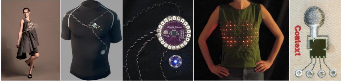
Figure 1.2: Applications making use of embroidered contacts (from left to right): the Climate dress with over hundred LEDs that visualize the CO 2 content of the surrounding air was designed for the climate conference in Copenhagen [12]; an EKG shirt with embroidered electrodes for measuring an electrocardiogram [13]; a do-it-yourself design kit with hand embroidered contacts [14]; shirt with LED display [15]; sensor for measuring an electromyogram [16].
