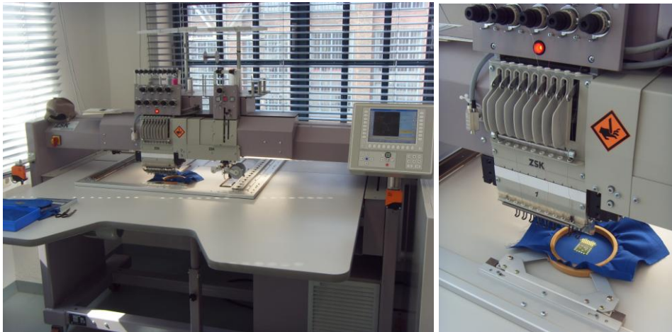
Figure 5.7: Embroidery machine ZSK JCZ 01 with regular embroidery head.
