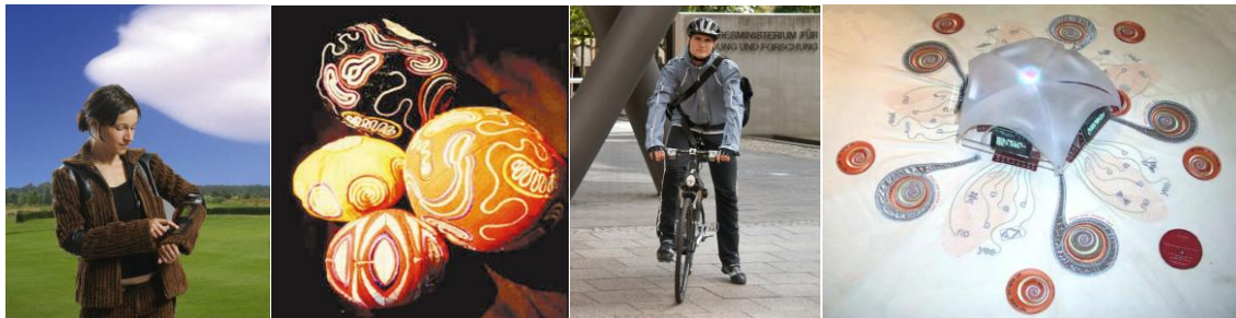
Figure 1.1: From left to right: communication jacket with arm wrist controls for a mobile phone in the pocket [4]; a performance art musical instrument with embroidered touch sensors [5]; a jacket for a bicycle messenger with integrated controls for navigation and managing job tasks [6]; interactive "board" game with embroidered user interface on tablecloth [7].
