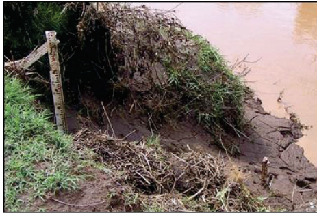
Figure 1.3: Staff gauge section at the Gumara station (source: SMEC, 2008). In this study, this station has been replaced by a new installation further downstream along this river.
