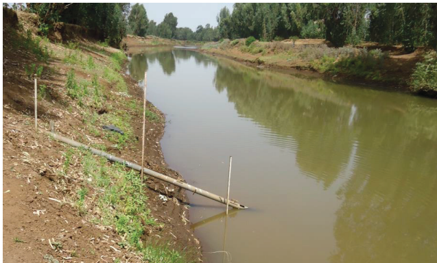
Figure 3.2: Typical monitoring station installation with staff gauges (vertical poles) and a pipe containing a Mini-Diver, at the deepest point of the river cross-section (Lower Gumara station, March 2012).
