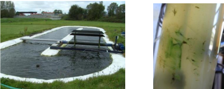
Fig. 1.5. Open raceway pond treating sewage (STOWA project, the Netherlands) (left) and biofilm fouling in wastewater treating closed photobioreactor (right)
