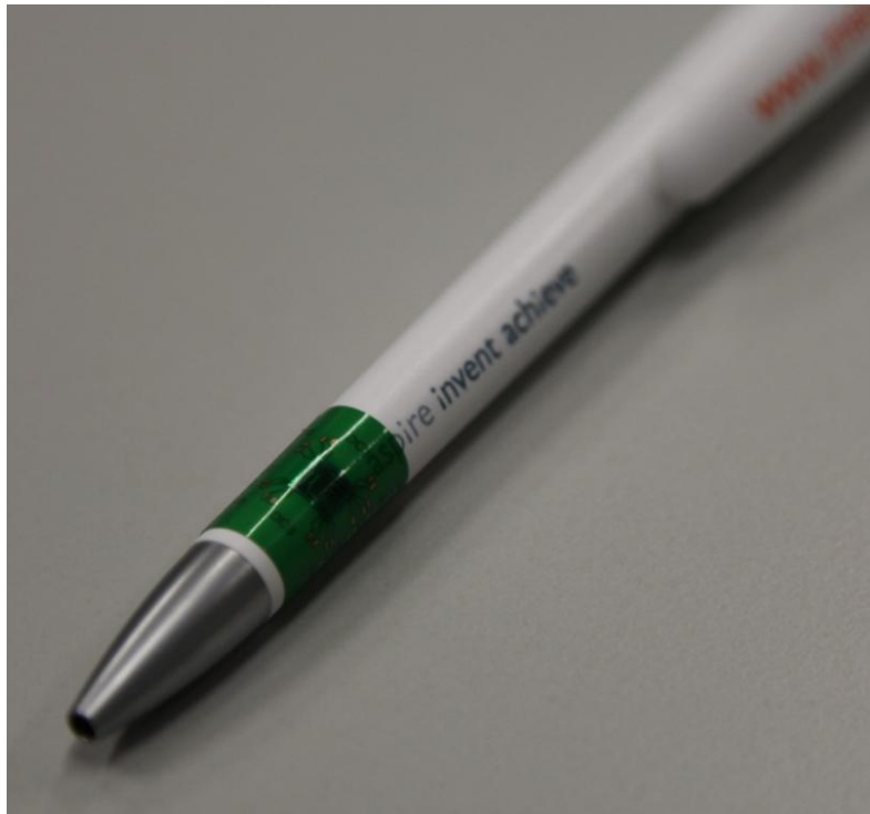
Figure 2.13 A realized UTCP bending around a pen to show its flexibility.
