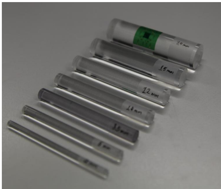
Figure 2.16, A UTCP is bent over on the surface of cylinders with diameter from 20 to 4 mm for mechanical flexibility test.
