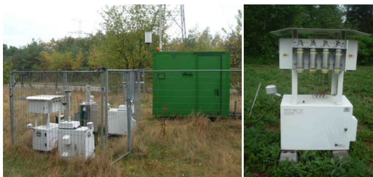
Picture 7: Sampling location and a Partisol speciation sampler used for the simultaneous sampling on 4 filters.
