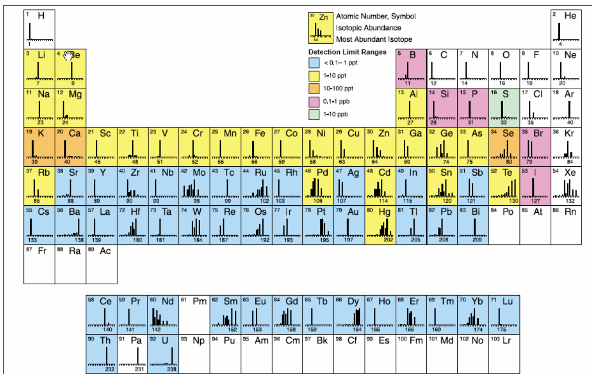
Figure 7: Approximate detection capabilities of the ELAN 6000 quadrupole ICP-MS (Courtesy of PerkinElmer, Inc.).
