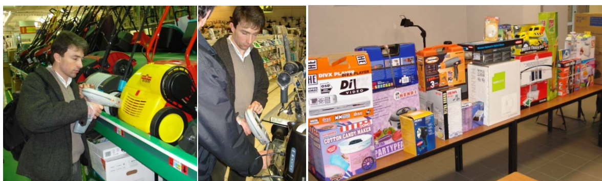
Picture 4: RoHS inspection campaign, electrical and electronic devices were (non-destructively) screened on-site in different electronic shops with EDXRF; 27 products were purchased and dismantled for further testing.
