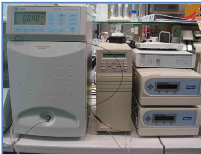
Picture 2: Ion chromatography instrument equipped with post-column derivatisation.
