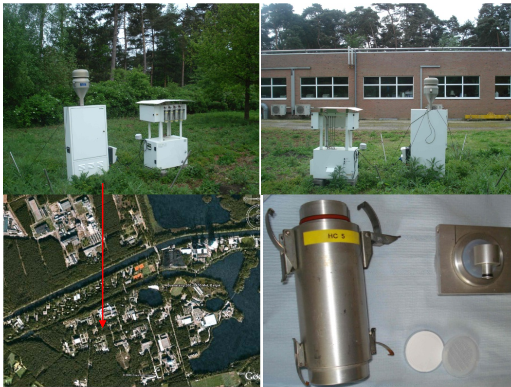
Picture 6: Digital DHA-80 high-volume samplers and Partisol speciation sampler in a rural area (Mol, Belgium), with details of the Partisol speciation sampler filter holder ( PM_{10} ).
