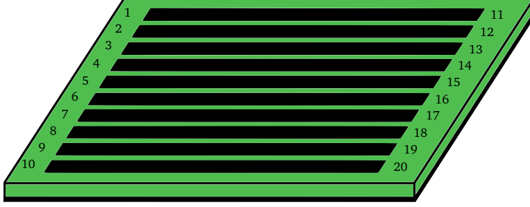
Figure 4.1: The nominal uniform microstrip line interconnection with ten signal conductors.
