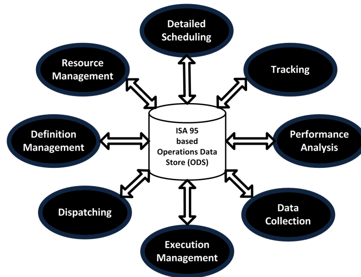
Figure 2.14: The use of one common ISA 95 based ODS ensures the integration of the MOM activities
