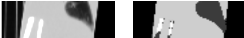
Figure 5.12: A sagittal slice of the CT-based (left) and UTE-MRI-based (right) attenuation map used for reconstructing the PET images of the thorax phantom.
