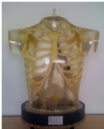
Figure 5.1: The Alderson phantom, a good example of an antropomorphic phantom used in PET, SPECT and CT.
