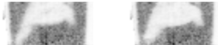
Figure 5.14: A coronal slice of the PET image of the thorax phantom reconstructed with CT-based (left) and UTE-MRI-based (right) attenuation correction.
