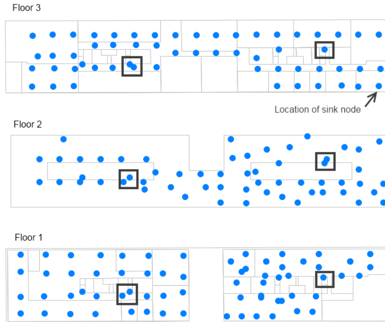
Figure 3.6: The ilab.t wireless sensor testbed contains about 200 nodes spread over 3 floors. Each floor measures 15 by 90 meter. The sensor nodes are indicated with a dot. Elevator shafts, indicated with a rectangle, provide connectivity between different floors.
