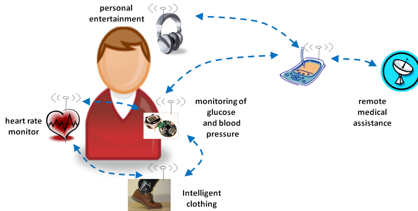
Figure 1.3: A body area network (BAN) can be used to monitor the life signs of patients so that a faster medical intervention is possible.
