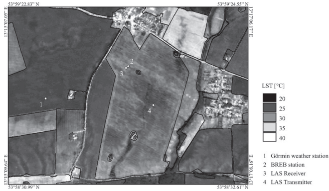
Figure 11.1: Station set-up in the winter-wheat field. The soil moisture observations are taken at the same location as the (BREB)-based observations [105].
