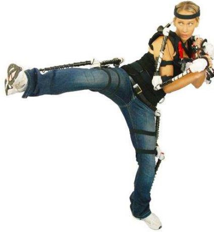
Figure 1.1: A person equipped with a mechanical tracking system.
