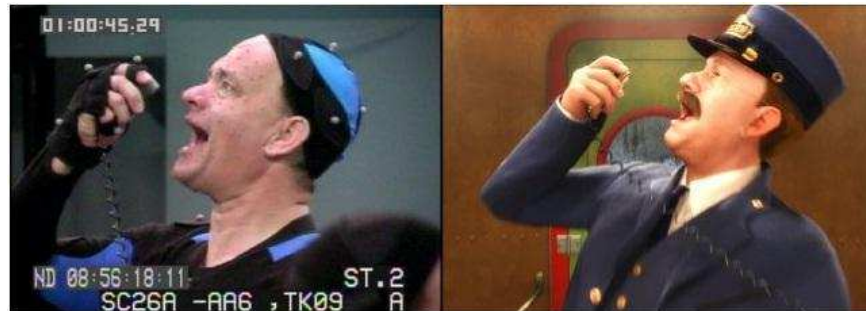
Figure 1.2: The posture of the person on the left is captured using an optical system and mapped to a computer generated character on the right.
