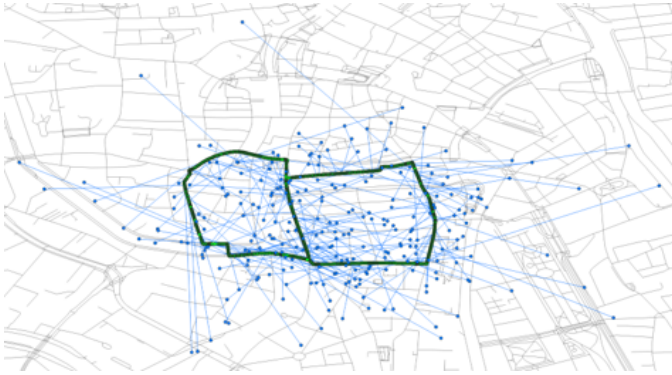
Figure 2: Ground truth (trace) and estimated TDoA locations (dots) from Semtech solver
