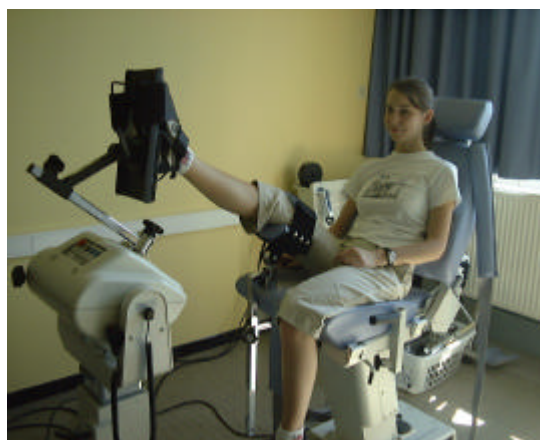
Figure 2. Positioning of the subject for testing isokinetic ankle inversion/eversion on the Biodex 3 isokinetic dynamometer
