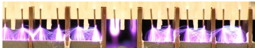
Figure 5.2 Photograph of the pulsed streamer discharge; the central needles are not connected.
