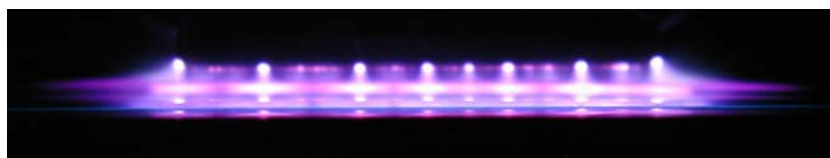
Figure 3.11 Photograph of the wedge-to-plate DBD in He + 2% \text{O}_2 at atmospheric pressure with f = 50 kHz and d = 2 mm.
