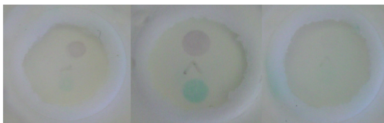
Figure 8.3: Result of a blond beer assay: anti-OTA antibodies and anti-DON antibodies spotted in dilution 1/10, 0.7 \mu\text{L} , OTA-AP-dilution 1/500, DON-HRP-dilution 1/2200, 5 mL blond beer sample, left side: no mycotoxins, middle: assay with buffer solution, right side: spiked sample, OTA, 2 \mu\text{g L}^{-1} , DON, 50 \mu\text{g L}^{-1}
