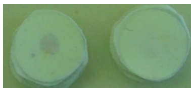
Figure 8.2: Result of a red wine assay: anti-OTA antibodies spotted in dilution 1/20, 0.7 \mu\text{L} , OTA-AP-dilution 1/500, 1 mL red wine sample diluted with 0.5 mL of salt solution, left side: no OTA, right side: spiked sample, OTA, 10 \mu\text{g L}^{-1}
