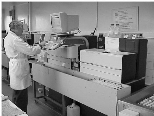
Figure 7. MilkoScan 4000 mid-infrared-photospectrometer (Foss Electrics) for the quantitative analysis of fat, protein and lactose in whole milk samples under accreditation circumstances (picture of MCC, Lier, Belgium).
