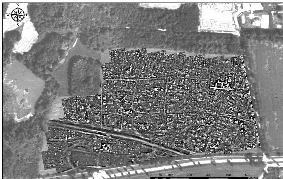
Figure 9.4: Results of large-scale high-resolution geomagnetic prospection conducted with a multi-sensor Caesium magnetometer superimposed within a GIS onto an aerial photograph. The dimension of the large field in the centre is 400 m (E–W) × 200 m (N–S). In the northern part the excavated ruins of the public baths are visible. Numerous streets, lanes and buildings can be seen as linear magnetic anomalies crossing this part of the civil town of Carnuntum. The wide linear anomaly in the SW is caused by the town fortification (rampart and trench); this structure and adjacent streets towards the N are as well visible in the vertical aerial photograph. The strong magnetic anomaly in the NE part of the central survey area is caused by thermoremanent magnetised structures of the forum of Carnuntum, stretching towards the baths in the north (ZAMG Archeo Prospections® and VIAS-University of Vienna).
