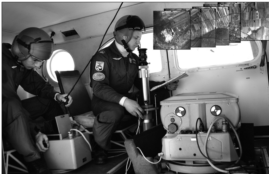
Figure 9.1: Series of panchromatic vertical aerial photographs taken by the Austrian Air Force with up to 60% overlap between images permit three-dimensional viewing and stereoscopic mapping (LBI ArchPro and Austrian Air Force, Fliegerstaffel Langenlebarn).
