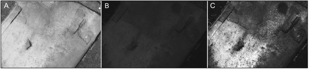
Figure 4.10 Comparison between a visible frame (A), unprocessed RAW NUV image (B) and enhanced NUV photograph (C) of an excavation area in Potentia. The large dark blob in the upper right corner of (B) and (C) is the shadow cast by the Helikite. The images were acquired with a Nikon D70s on July 05, 2008 at 12.06 h (A) and a Nikon D80 FS at 13.59 h on the same day (B–C) (Verhoeven and Schmitt 2010: fig. 12).
