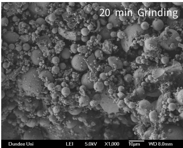
Figure 10. Scanning electron microscopy images of stockpile fly ash: SFA1 (top left) and after ball milling for 10 min (top right), 20 min (bottom left) and 30 min (bottom right)
