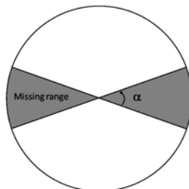
Figure 4.37: The missing angular range in a limited angle tomography.
