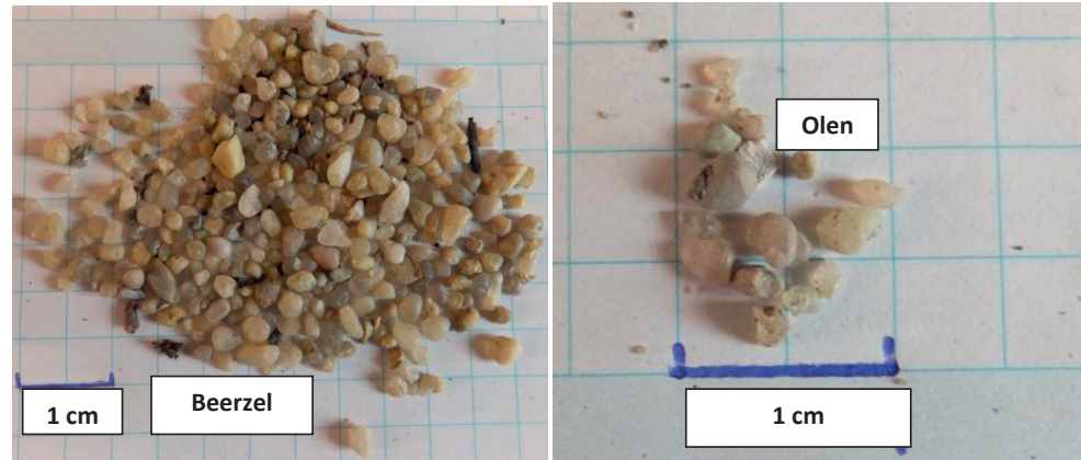
Figure 9. Pictures of the angular quartz grains present both in the basal gravel at Beerzel and Olen.
