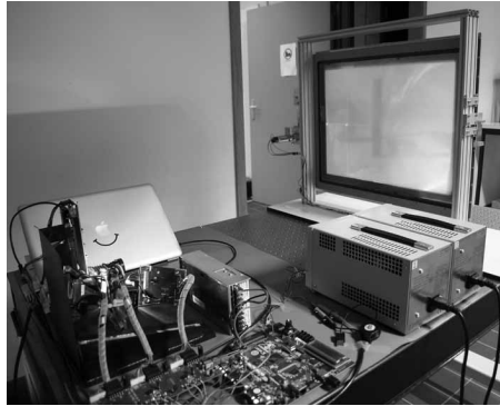
Fig. 8. Picture of the prototype system. The projector is located on the left and the image steering projection screen on the right. The 3D images are seen on the other side of the projection screen (Media 1).
