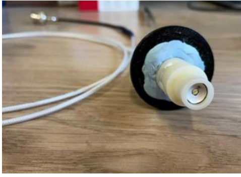
Fig.1 HIFU transducer made by Chongqing HAIFU company.
