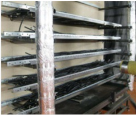
Fig. 1 The five horizontal cable tray device used for the CFSS fire tests
