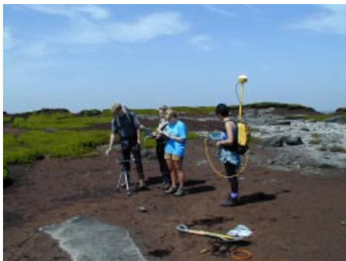
Plate 2: Collecting peat spectra with an ASD Fieldspec Pro spectroradiometer.
