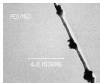
Figure 2. High-resolution TEM image of a single MgO nanoparticle embedded on the surface of a PEO nanofiber [3, 6].
