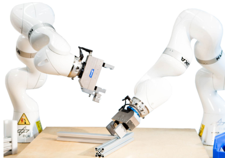
Figure 1.1.: A two-arm robotic system, similar to the one simulated by our environment, assembling a metal structure (Rodriguez et al., 2020).
