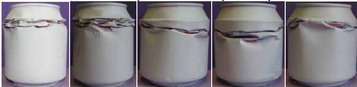
(b) Deformation patterns for initial impact velocity 2.2 m/s
