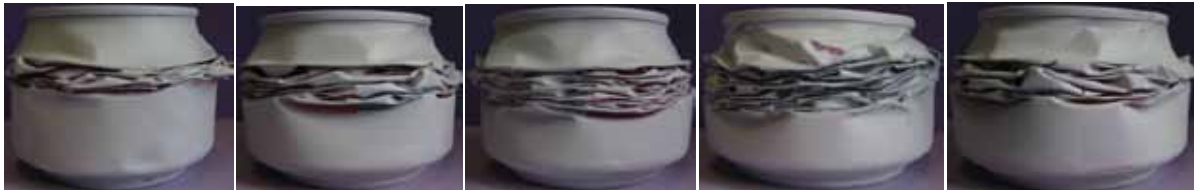
(e) Deformation patterns for initial impact velocity 4.4 m/s
