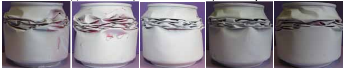
(c) Deformation patterns for initial impact velocity 3.1 m/s
