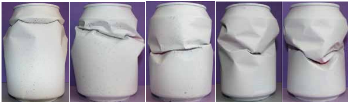
(a) Deformation patterns for initial impact velocity 1.4 m/s
