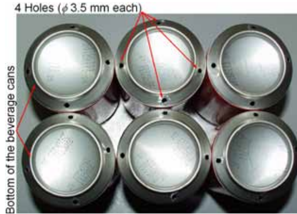
Figure 15: Beverage cans with holes at the bottom (to remove the air inside the beverage can during the crushing process).
