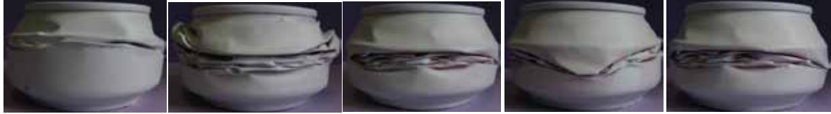
(f) Deformation patterns for initial impact velocity 4.9 m/s
