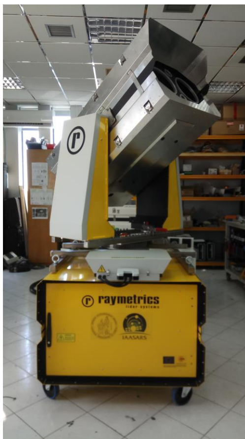
Figure 7. The WALL-E polarization lidar system for the detection of preferential particle orientation.
