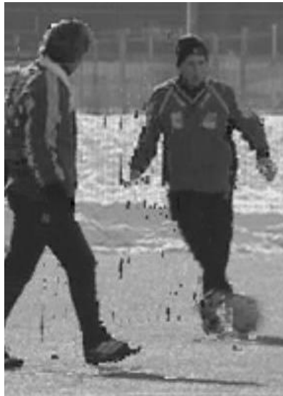
(a) Open-loop transcoding (detail of Soccer , QP 22, 4CIF to CIF, 9th frame).
