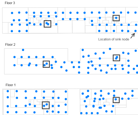
Figure 6: The W-ilab.t wireless sensor testbed contains about 200 nodes spread over 3 floors. Each floor measures 15 by 90 meter. The sensor nodes are indicated with a dot. Elevator shafts, indicated with a rectangle, provide connectivity between different floors.
