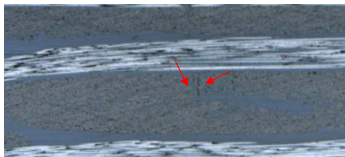
Damage location at 2-1(nested yarn)
