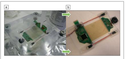
**Figure 7.** Stretchable molded interconnect circuit (a) during and (b) after the liquid injection molding process.<sup>8</sup> Device size is  $\sim$ 5 × 8 cm<sup>2</sup>.
