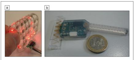
Figure 11. (a)  $7 \times 8$  light-emitting diode matrix (device size is  $\sim 9 \times 9$  cm<sup>2</sup>); (b) wireless electrocardiogram monitor with stretchable antenna and interconnect to distant electrode.24 Note: A one Euro coin is included for scale.
