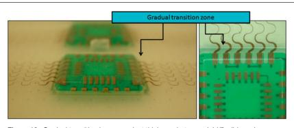
Figure 10. Gradual transition in encapsulant thickness between rigid/flexible and stretchable zones avoids local stress concentrations in the transition area.<sup>8</sup>
