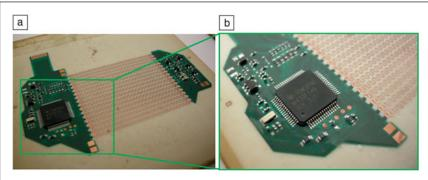
**Figure 5.** Assembled stretchable molded interconnect circuit on a temporary carrier: (a) overview and (b) detail.<sup>8</sup> Device size is  $\sim 5 \times 8$  cm<sup>2</sup>.
