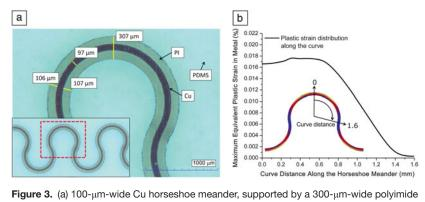
layer; (b) plastic strain distribution along the supported meander at a uniaxial stretching of 40%.<sup>15</sup> Note: PDMS, polydimethylsiloxane; PI, polyimide.
