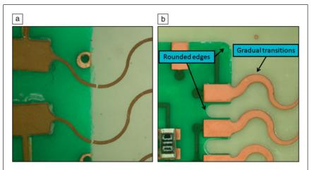
Figure 9. (a) Non-optimized and (b) optimized design at a transition area between rigid/flexible and stretchable zones. Gradual transitions in width of the copper and corresponding supporting polyimide reduce the local plastic strain in the copper. Sharp edges need to be omitted.<sup>8</sup> Copper track width is ~100  $\mu$ m.
