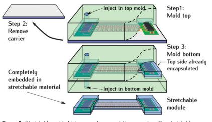
**Figure 6.** Stretchable molded interconnect encapsulation procedure: The stretchable circuit adhering to the temporary carrier is partly encapsulated by injection molding the polymer on top of the circuit. After curing the polymer, the temporary carrier is removed, including the temporary adhesive. A second molding step takes place in order to fully encapsulate the device in a stretchable polymer.<sup>8</sup>
