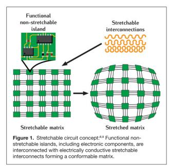
rigid component islands and the stretchable meander copper conductors (see the section on Mechanical modeling and design) is extremely important for obtaining a desired level of mechanical reliability (i.e., under cyclic stretching) of the circuit. As a general rule, a gradual transition from rigid to flexible to stretchable is necessary to obtain a mechanically reliable circuit.
