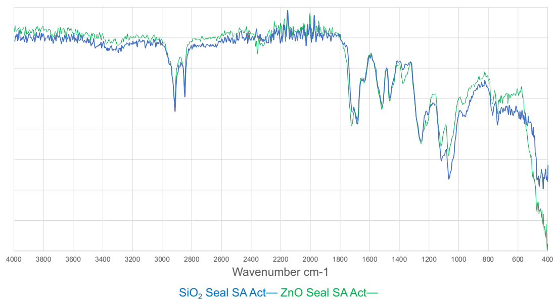
Figure 4-5 Transmission FT-IR spectra of two Altro Seal coating. The coatings contained either ZnO or SiO 2 , as well as Altro Seal (Seal), stearic acid (SA), and was made up in acetone (Act)
