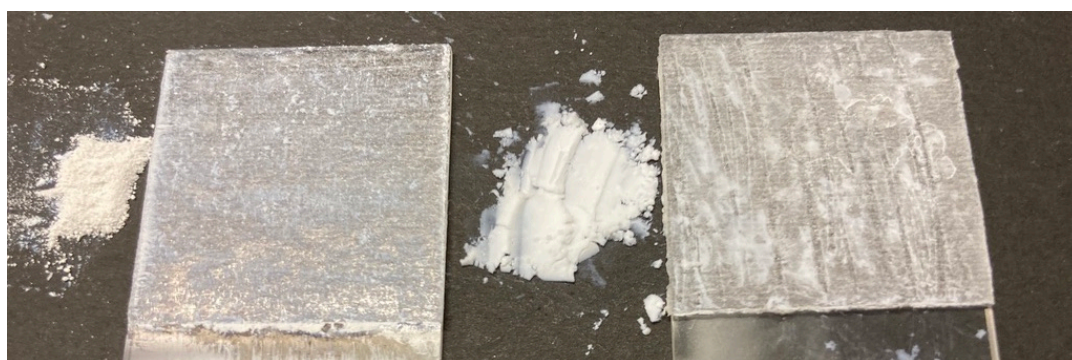
Figure 3-2 Functionalised ZnO powder (left powder). Functionalised ZnO powder on double sided tape (left). Functionalised SiO 2 powder (right powder). Functionalised SiO 2 powder on double sided tape (right)
