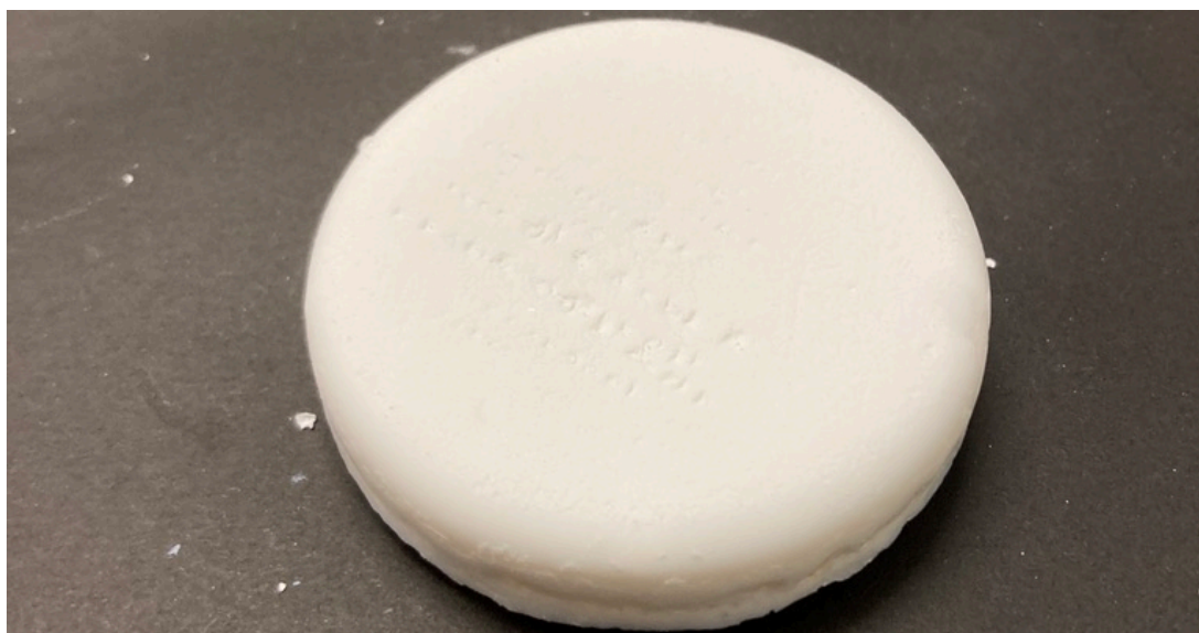
Figure 5-6 Bulk polyurethane fabricated using a similar formulation to the superhydrophobic Altro Seal coatings (section 4.3.2)
