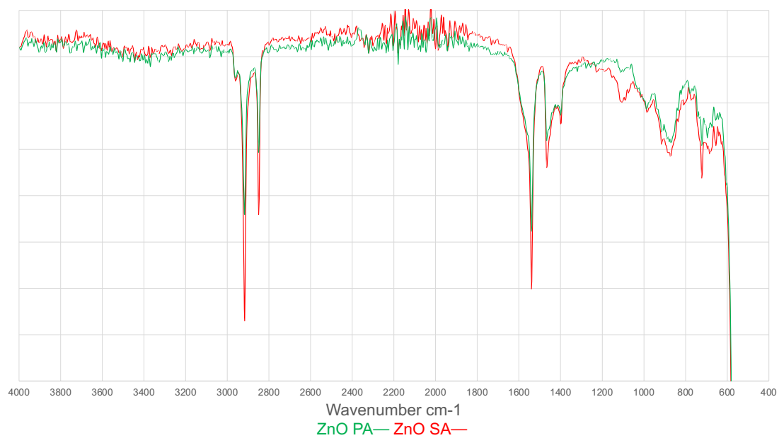
Figure 3-12 The comparison of the transmission FT-IR spectra of ZnO functionalised with stearic acid in acetone and ZnO functionalised with palmitic acid in acetone.
