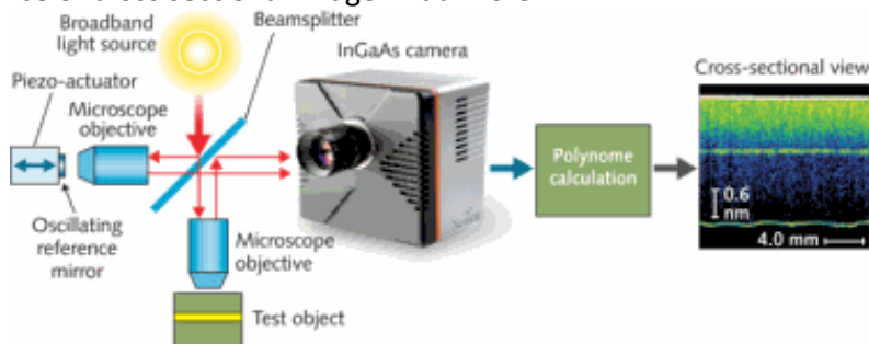
Figure 4: Full-field OCT with a very fast 2D camera Cheetah-640 CL (MO = microscope objective)
