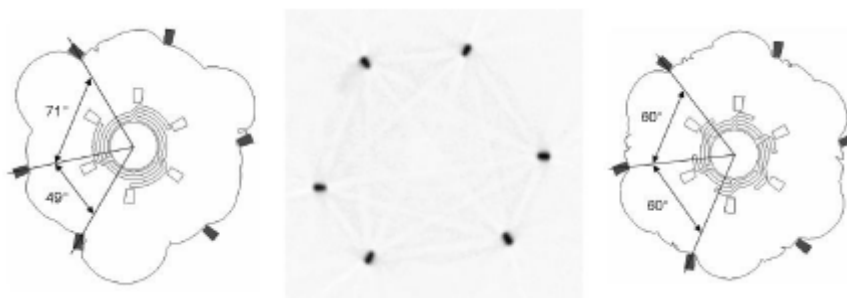
Figure 2: For the trifolded balloon, a non-uniform stent strut distribution was observed (left panel: simulation; center panel: experiment), whereas a six-folded balloon (right panel: simulation) results in a homogeneous strut distribution.
