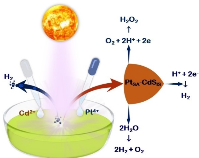
Scheme 1. Cooperative coupling of solar H 2 generation and in situ synthesis of Pt single-atom anchored CdS 15 nanoparticles (Pt SA -CdS 15 ) during photoirradiation. Schematic illustration highlighting the concurrent H 2 production and synthesis of Pt SA -CdS 15 semiconductors in a single photoinduced reaction system.
