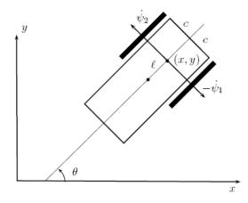
The angle of rotation about the vertical is denoted by  $\theta$ , and the positions of the wheels are characterized by angles  $\psi_1$  and  $\psi_2$ . We shall generally assume that the intersection point (x, y) of the horizontal symmetry axis of the carriage with the line which connects the two wheels is not necessarily the centre of mass of the system, but lies at a distance  $\ell$  from it.
