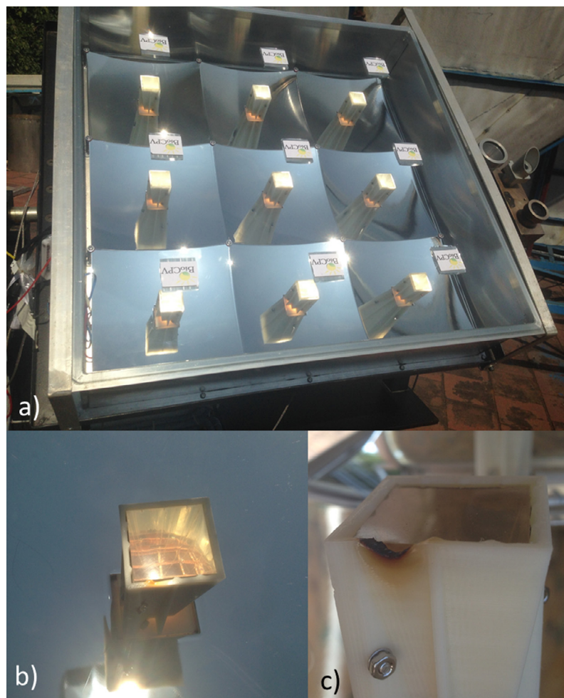
Fig. 8. (a) Photo of complete 3 by 3 prototype with side walls in place (closed) mounted on a 2 axis automatic tracker at IIT Madras, Chennai. (b) Photo of CRRH with concentrated light focusing off-centre onto plastic material of 3d printed support structure and causing burn marks. (c) Close up photo of melting due to >20 min of focused light incident on CRRH plastic support structure.
