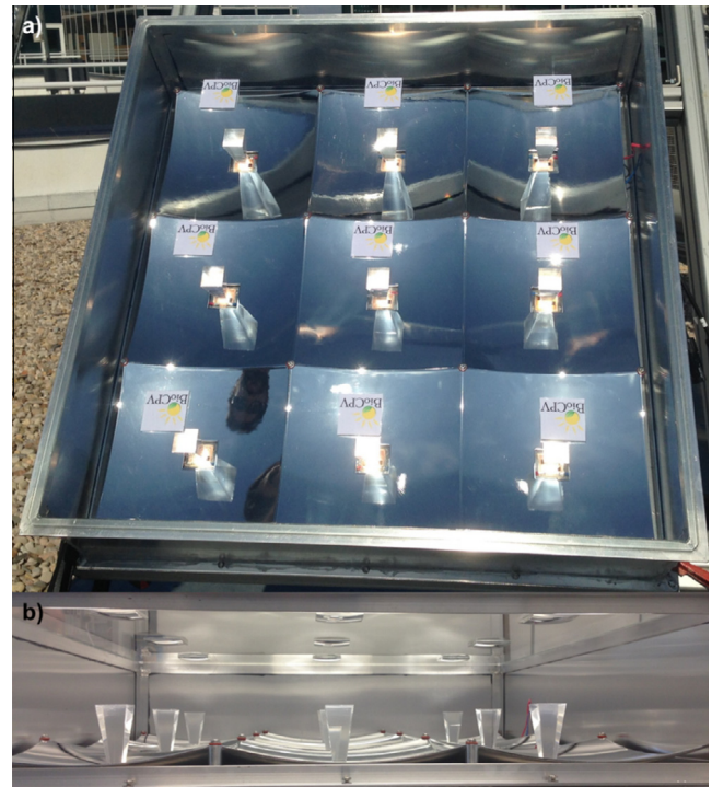
Fig. 10. Photo of 3 by 3 cassegrain concentrator prototype from (a) top view and (b) side view. (a) Shows the concentration of sunlight onto the homogenisers and solar cells.
