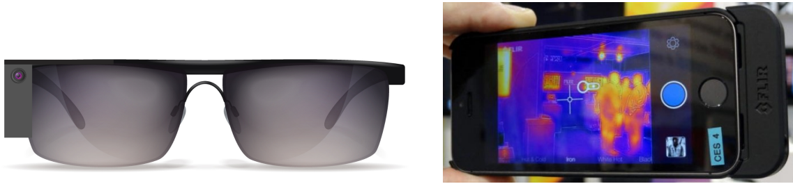
Fig. 1. Examples of how thermal cameras are becoming more portable, discrete and usable in everyday scenarios Left: Illustration of possible future wearable thermal camera, based on current research prototype [10]. Right: Thermal camera smartphone add-on [13].
