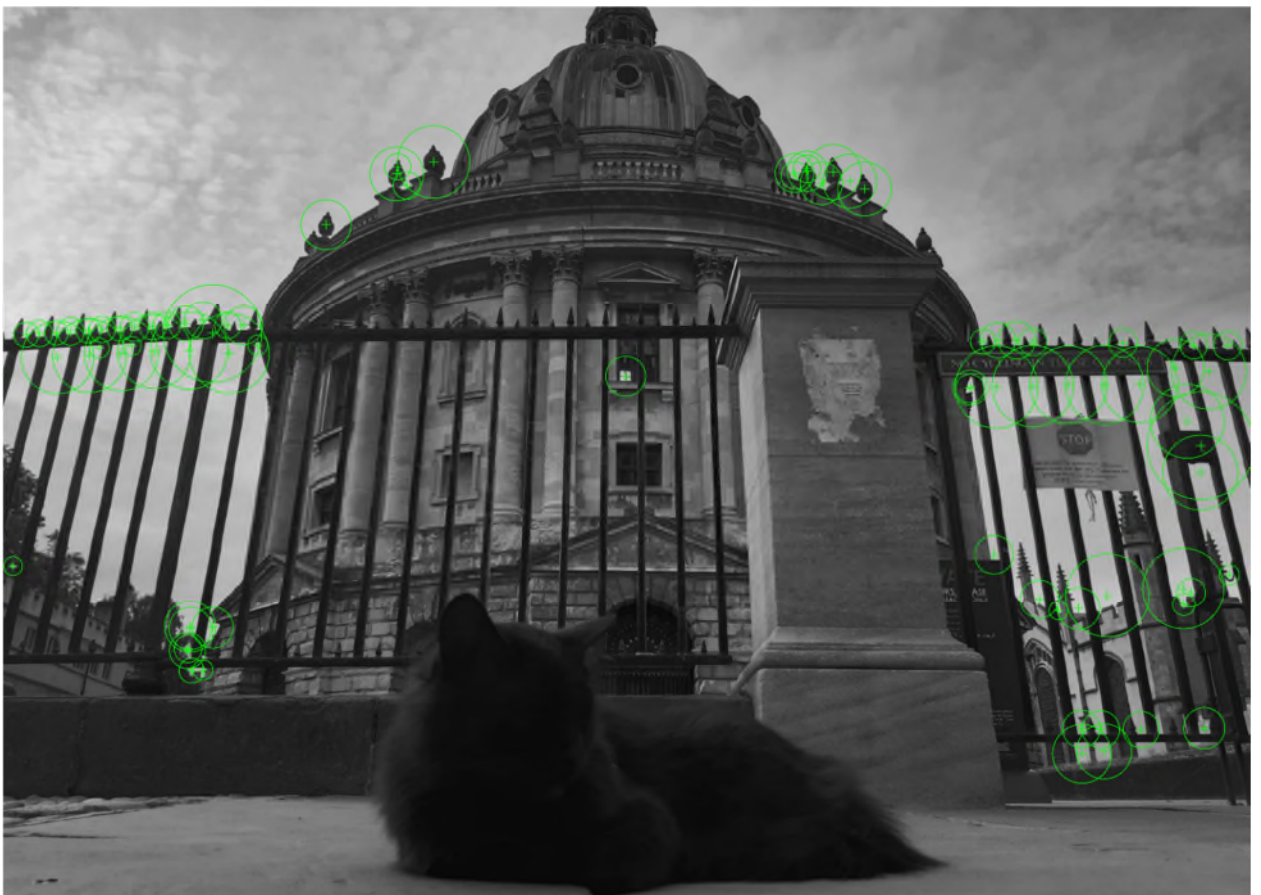
Figure 5-12 - The 80 strongest SURF features (green crosses and circles) detected within the underlying image.
