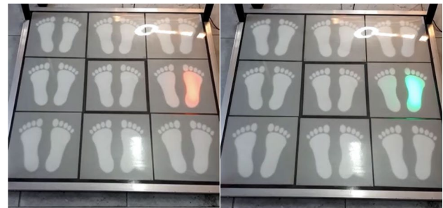
Fig. 3 Red led: target led; and green led: confirmation led
