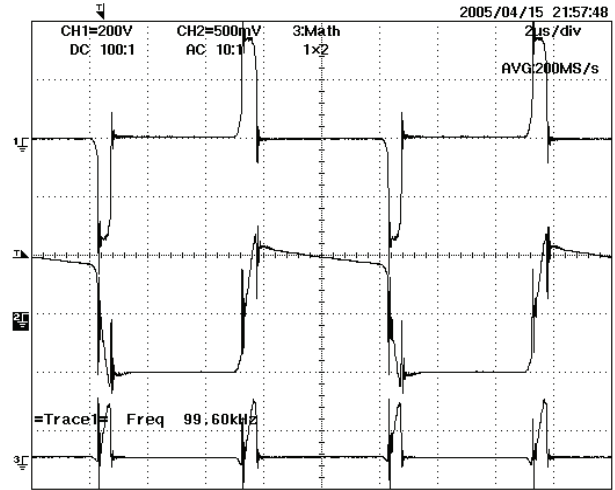
Fig.4. Measured Voltage, current and power for a full bridge at D=0.05, 200V/div 500mA/div, 100W/div
