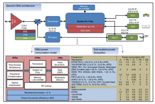
Fig. 1. ONU power consumption model.
