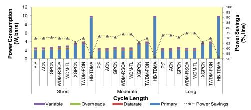
Fig. 4. Power Consumption (W) of various NGOA systems in doze mode during busy hours with three values of the cycle length: short (5 ms), moderate (20 ms) and long (100 ms). The bars representing variable, overheads, and data rate components will be zero for the best case scenario.
