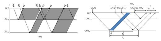
Fig. 2. (a) A TDMA-PON with an OLT and two ONUs showing REPORT (R1 and R2 for ONU1 and 2) and GATE (G1 and G2 for ONU1 and 2) messages transmission. (b) GATE prediction in the SMA algorithm.
