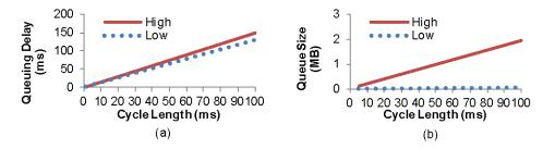
Fig. 6. (a) Queuing delay vs. cycle length (b) Queue size vs. cycle length. H (high = 100 Mbps) and L (Low = 1.5 Mbps) data rates are evaluated.
