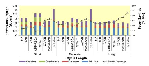
Fig. 5. Power Consumption (W) of various NGOA systems in sleep mode during busy hours with three values of the cycle length: short (5 ms), moderate (20 ms) and long (100 ms). The bars representing variable, overheads, and data rate components will be zero for the best case scenario.
