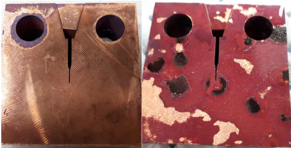
Figure 18. Left: bottom surface and Right: top surface of the specimen after the 5000 hour exposure.
