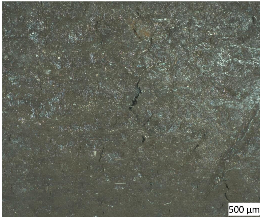
Figure 6. Oxide cracks in the specimen y211 after 170849 hours.
