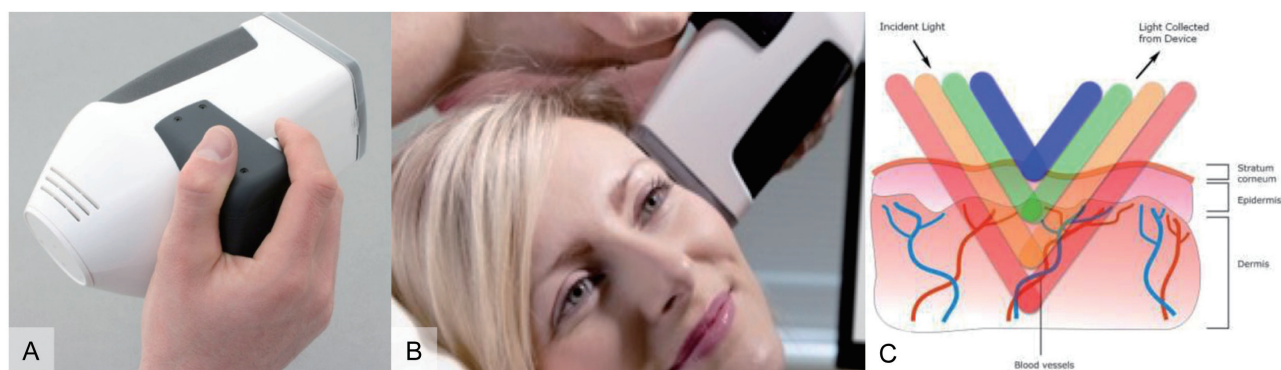
Fig. 1. Antera 3D®. (A) Photograph showing the size and portability of the Antera 3D® device. (B) The 5.6 × 5.6 cm flat surface of the device is placed against the skin for imaging. (C) Diagram shows the application of visible light LED to the skin surface from multiple directions to analyze the concentration and scatter of hemoglobin. All images were sourced from Miravex Limited with the permission. LED, Light Emitting Diode.
