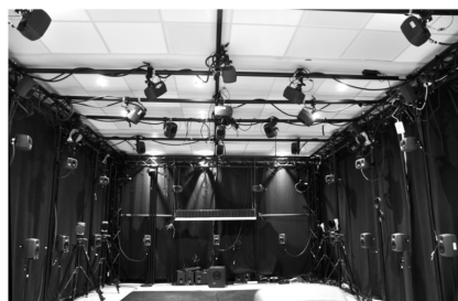
(a) 47-loudspeaker 3-D array at the motion capture lab at the Department for Musicology, University of Oslo.
