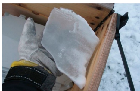
Figure 3. Ice piece thrown from a WT in Arctic Norway WF [36]. Reprint with permission from author [Matthew Homola], 2022, NTNU Norwegian University of Science and Technology.
