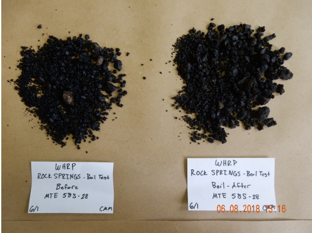
Figure B-10 Before and after boil testing: Rock Springs aggregate with MTE 58S-28 binder
