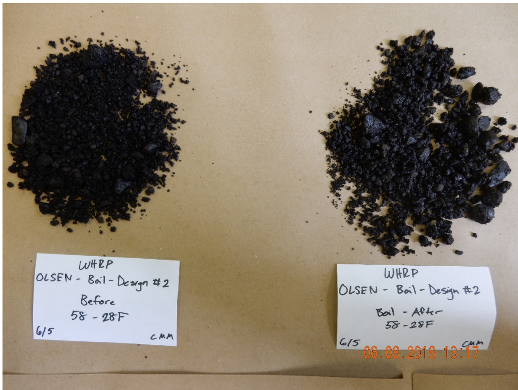
Figure B-15 Before and after boil testing: Olsen aggregate with 58-28F binder
