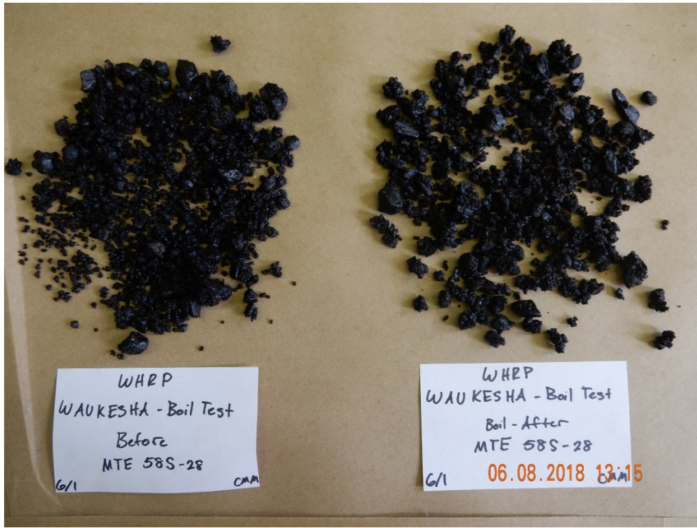
Figure B-2 Before and after boil testing: Waukesha aggregate with MTE 58S-28 binder
