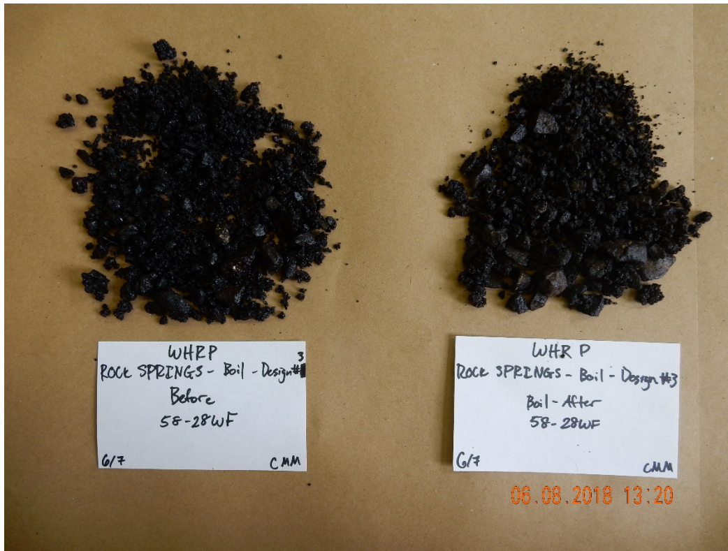
Figure B-12 Before and after boil testing: Rock Springs aggregate with 58-28WF binder
