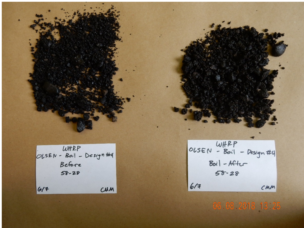
Figure B-17 Before and after boil testing: Olsen aggregate with 58-28 binder
