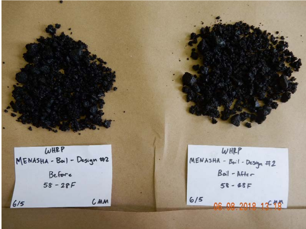
Figure B-7 Before and after boil testing: Menasha aggregate with 58-28F binder
