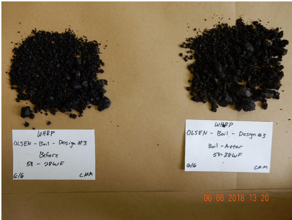
Figure B-16 Before and after boil testing: Olsen aggregate with 58-28WF binder
