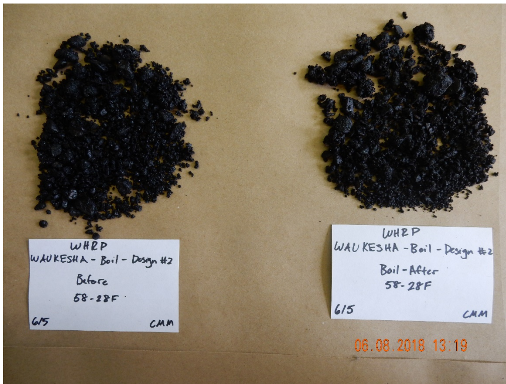
Figure B-3 Before and after boil testing: Waukesha aggregate with 58-28F binder
