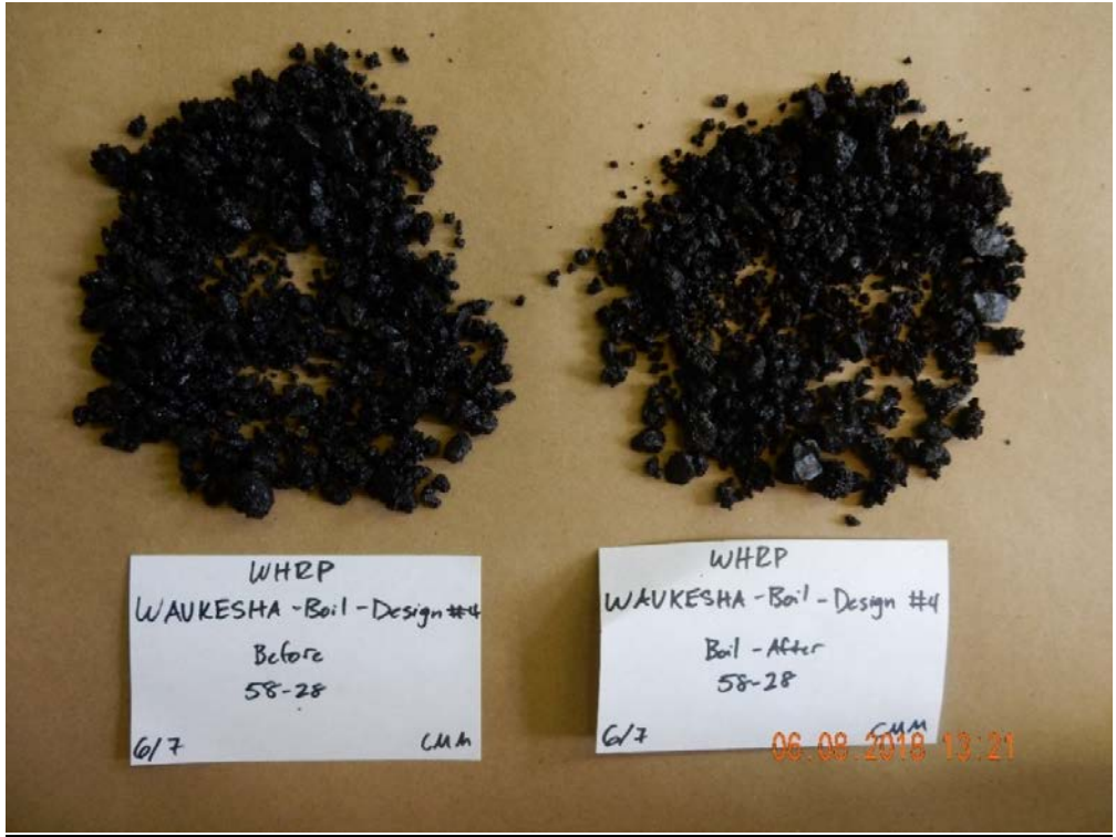
Figure B-5 Before and after boil testing: Waukesha aggregate with 58-28 binder
