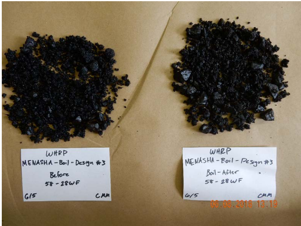
Figure B-8 Before and after boil testing: Menasha aggregate with 58-28WF binder
