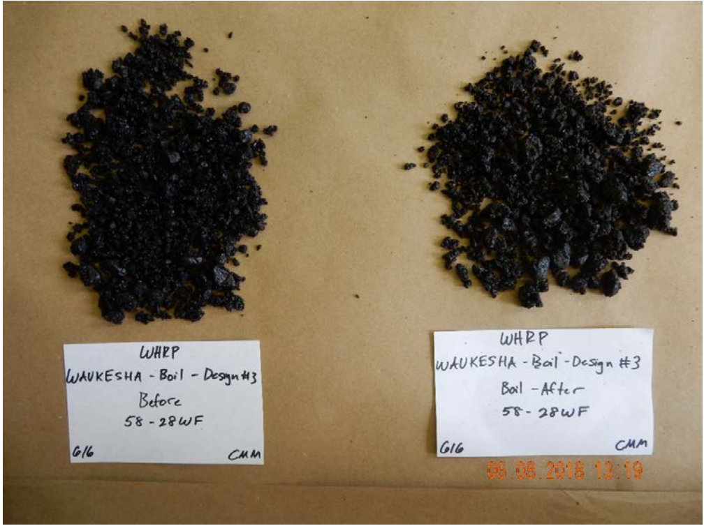
Figure B-4 Before and after boil testing: Waukesha aggregate with 58-28WF binder
