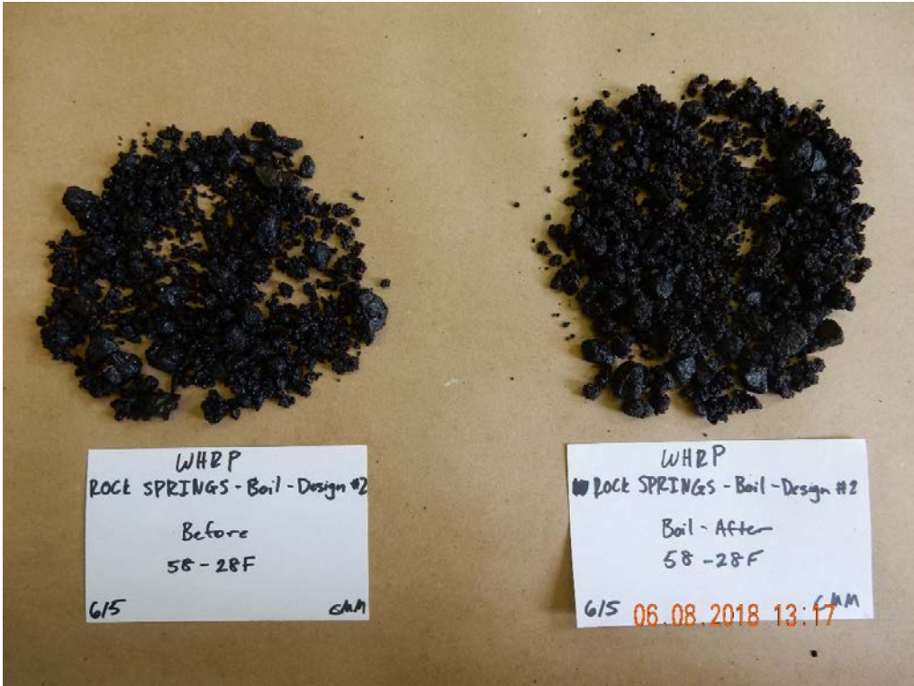
Figure B-11 Before and after boil testing: Rock Springs aggregate with 58-28F binder
