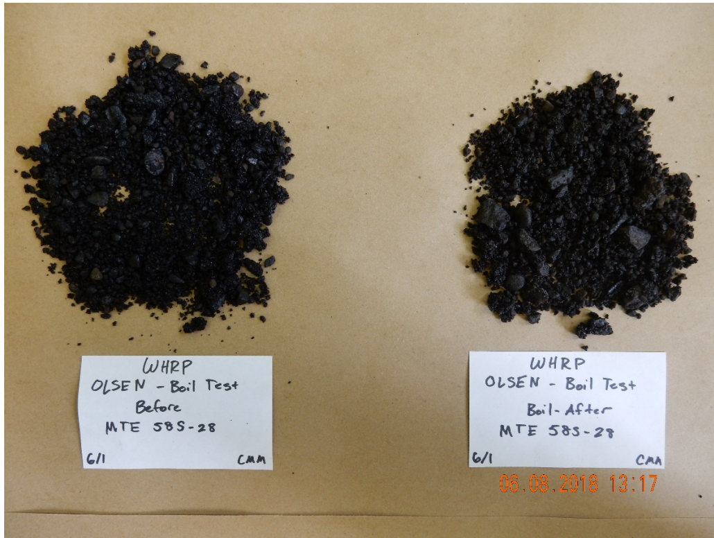
Figure B-14 Before and after boil testing: Olsen aggregate with MTE 58S-28 binder
