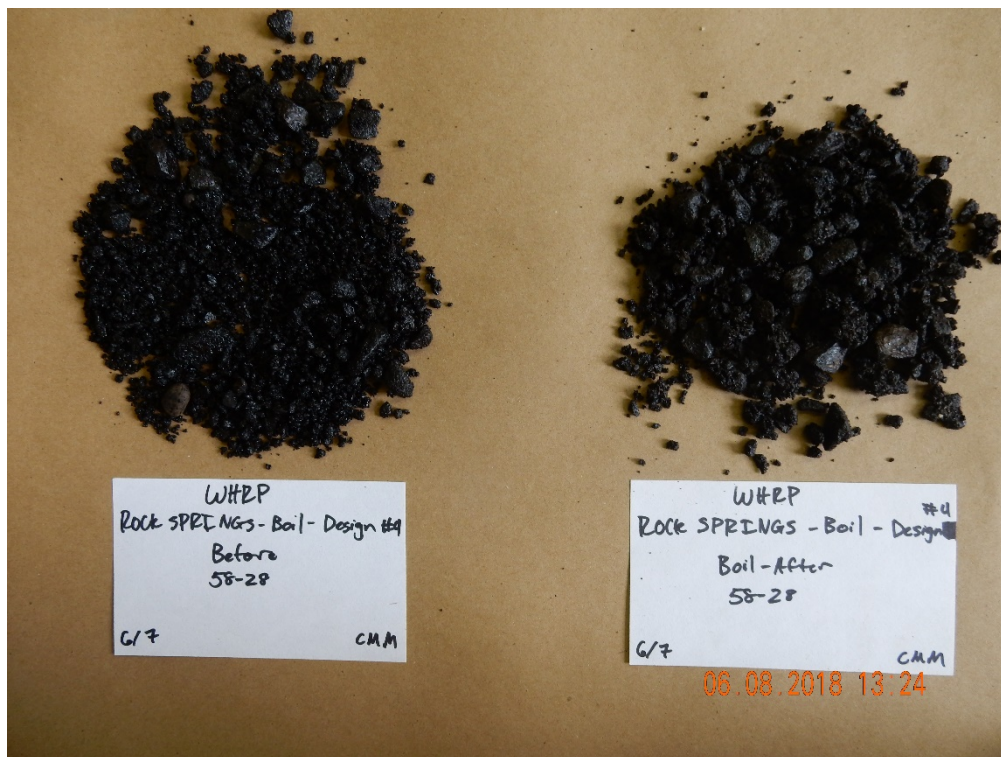
Figure B-13 Before and after boil testing: Rock Springs aggregate with 58-28 binder
