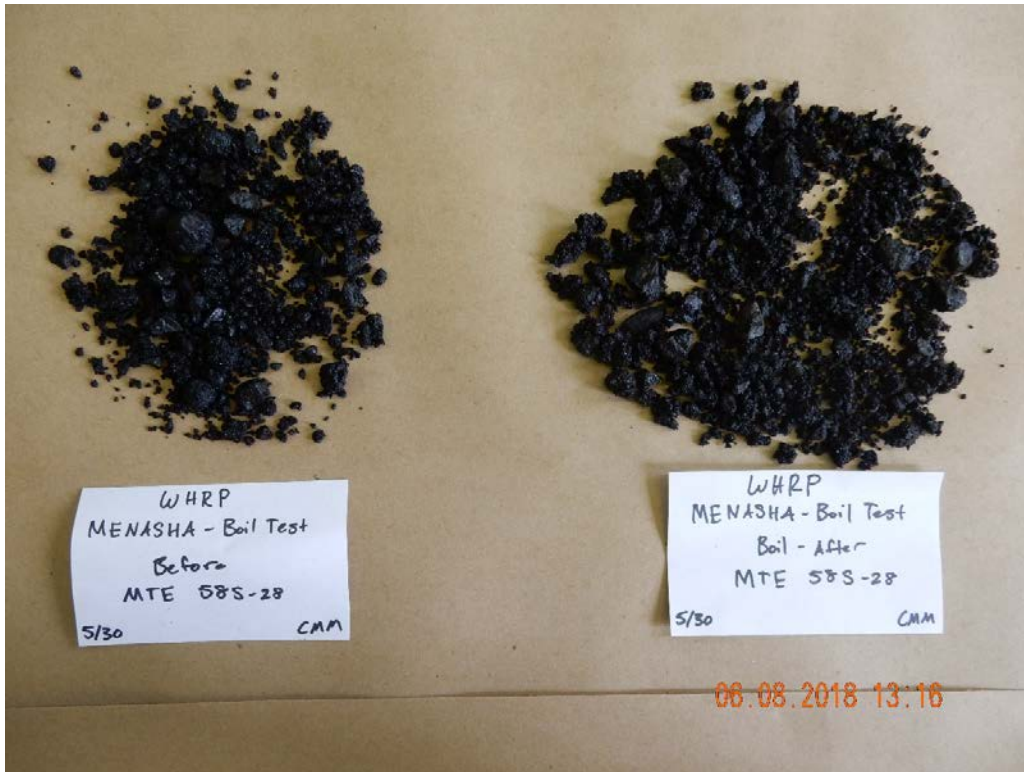
Figure B-6 Before and after boil testing: Menasha aggregate with MTE 58S-28 binder
